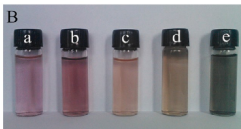
Figure 4. (A) UV–vis absorption spectra of PPyNT-Im-Pt 8 Au 2 , PPyNT-Im-Pt 5 Au 5 , PPyNT-Im-Pt 2 Au 8 , and PPyNT-Im-Au hybrids dispersed in water. (B) Photograph of colloidal aqueous solution containing 0.1 mM (a) PPyNT-Im-Au, (b) PPyNT-Im-Pt 2 Au 8 , (c) PPyNT-Im-Pt 5 Au 5 , (d) PPyNT-Im-Pt 8 Au 2 , and (e) PPyNT-Im-Pt hybrids.
